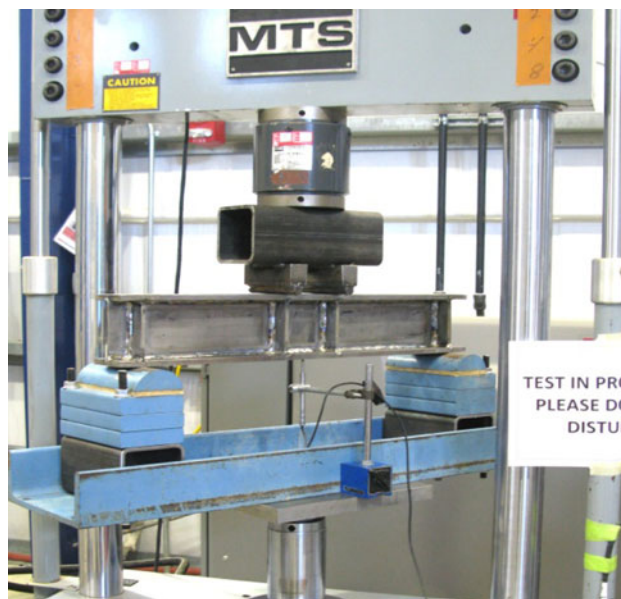
Fig. 5 The test set-up for the fatigue tests
